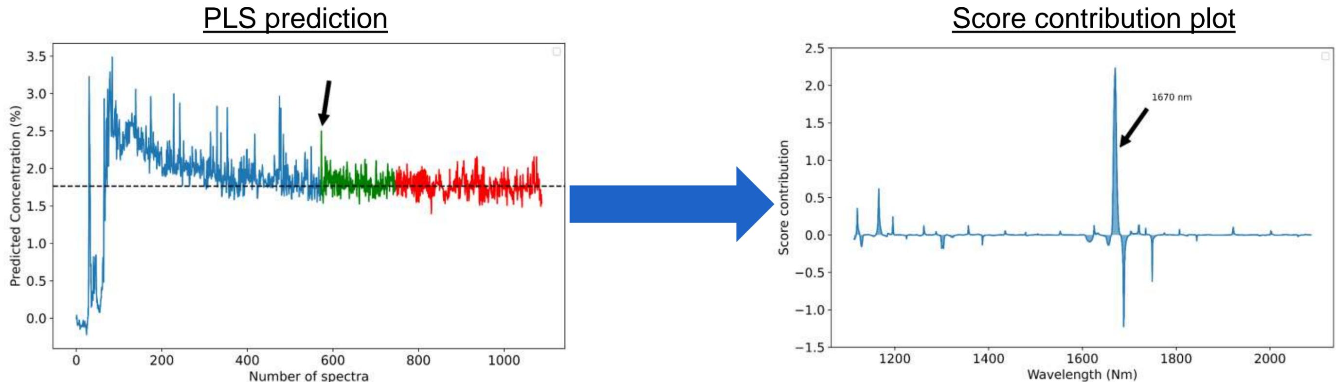
Fig. 12: Validation run of PLS model (7.5L-60RPM-B). Green coloring denotes a homogeneous powder mixture, which continues as red during the final two minutes of blending.
