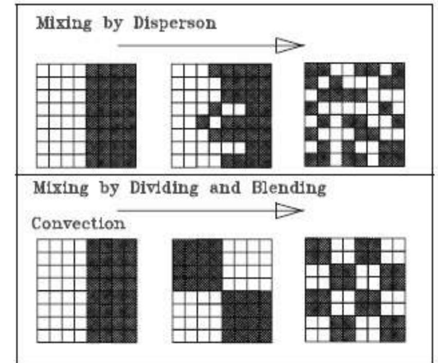
Fig. 3: Schematic overview of dispersive mixing (top) and convective mixing (bottom)
