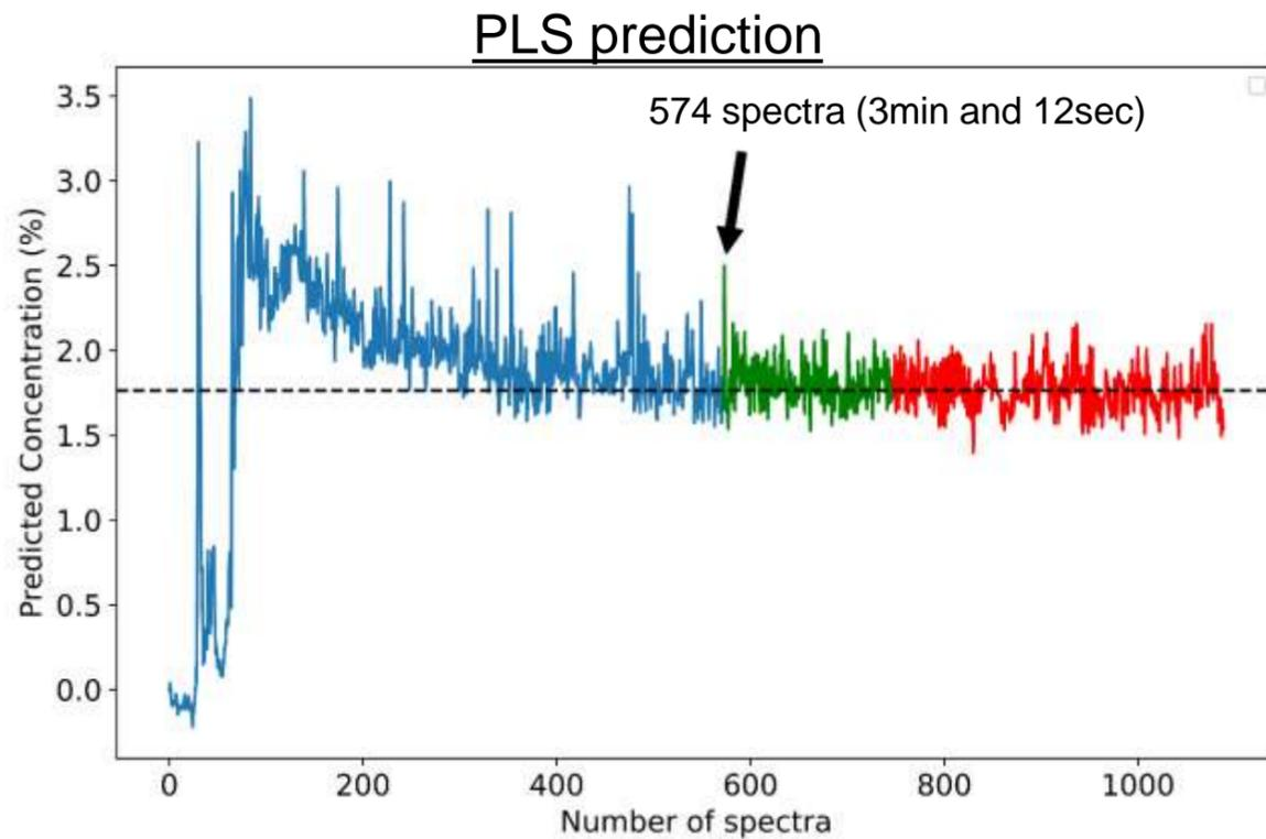
Fig. 12.: Validation run of PLS model (7.5L-60RPM-B). Green coloring denotes a homogeneous powder mixture, which continues as red during the final two minutes of blending.
