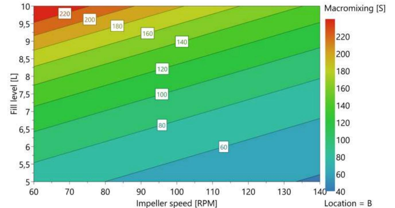
Fig. 24: Contour plot of the endpoint of macromixing
