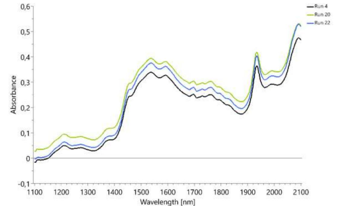
Fig.8: Raw spectrum of run 4, 20 and 22 collected during the final two minutes of blending
