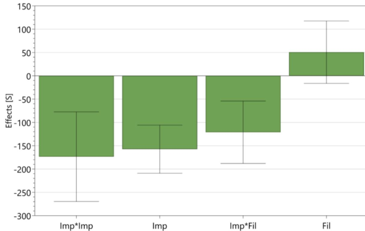
Fig. 25: Effect plot of micromixing. Imp: impeller speed, Fil: fill level
