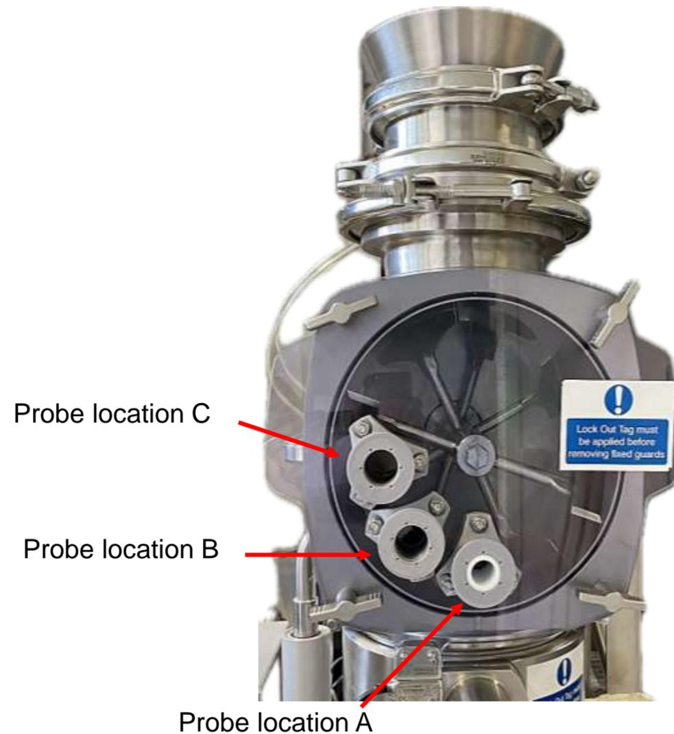
Fig. 2: Semi-continuous blender (GBM 10-P, Gericke AG)
