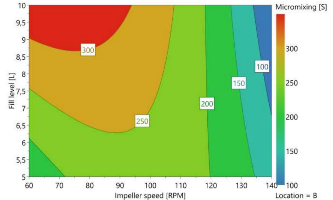
Fig. 26: Contour plot of the endpoint of micromixing
