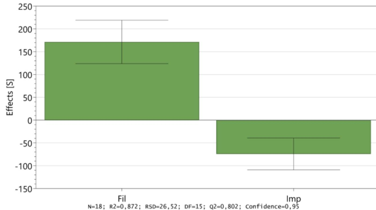
Fig. 23: Effect plot of macromixing. Imp: impeller speed, Fil: fill level
